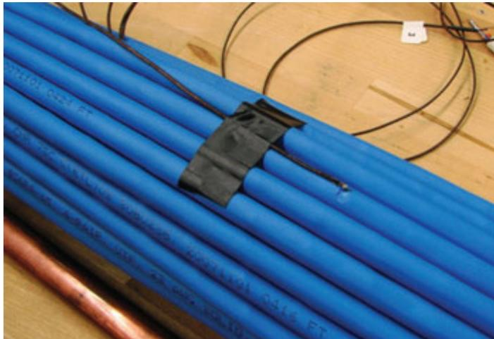
4. The finished 100-around-1 bundle was suspended in air at a minimum distance of 0.3 m from any object in all directions. The ends of the bundle were covered with insulating foam to eliminate heat dissipation from the ends of the bundle, thereby ensuring worst case heat build-up. Test leads from a continuous current power supply were attached to all 4-pairs in the cable bundle.
